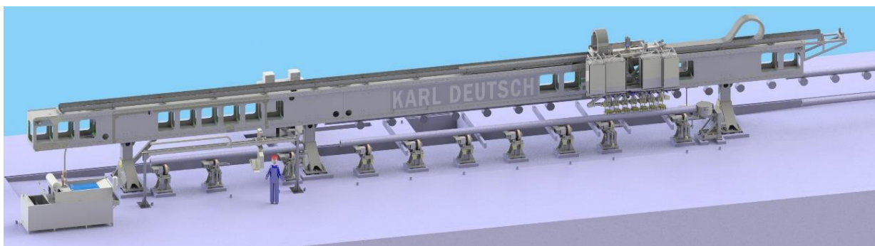
Fig. 2 High-Speed Tube Testing Portal with a length of 32 m.
