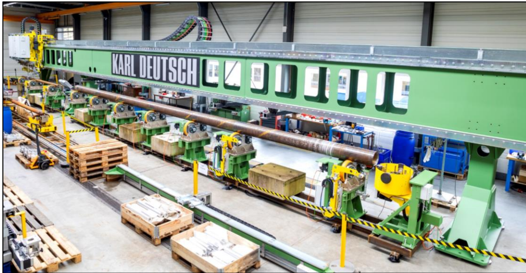
Fig. 3 Assembled tube testing system before shipment
