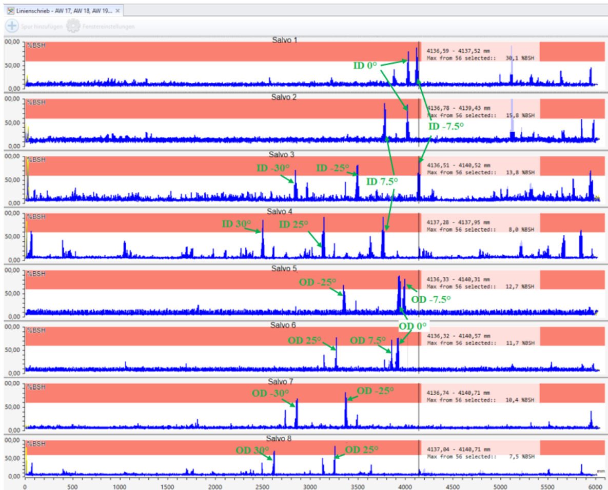
Fig. 13 Example of \pm 30^\circ flaw detection (probe cluster 1) in heavy-walled reference tube
