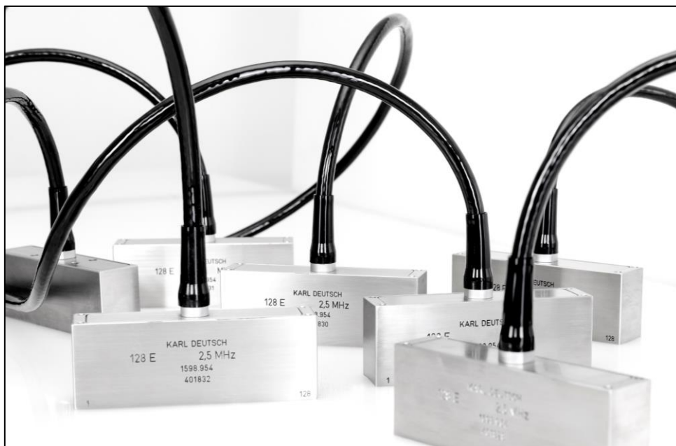
Fig. 6 PAUT Probes for seamless tube testing.
